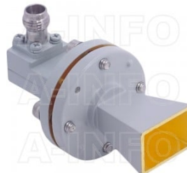
LB-19-15-C-2.4F Standard Gain Horn Antenna 40-50GHz 15dB Gain 2.4mm Female
