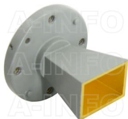
LB-19-15-A Standard Gain Horn Antenna 40-60GHz 15dB Gain Rectangular Waveguide Interface
